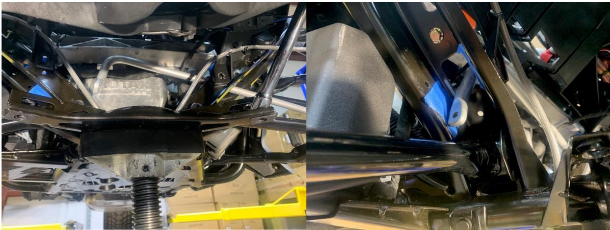
10.- Then install the sets of Sway Bar bushings using the factory bolts. The bushings go in one direction only. The top of the bushings has chamfered cuts to allow them fit in the upper frame channel. Notice the bushing is in two parts you want the hole that is angled to be towards the back with the thicker side of the bushing facing the front of the Ryker as shown below. Do this on bolt sides. Do not tighten down all bolts until all bolts are in their locations.
