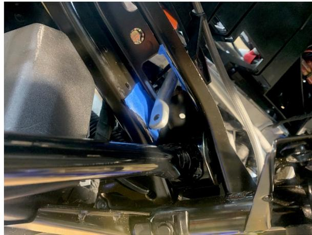
7.- Then the wiring harness below and cut the two wire ties and place the harness under the tabs in red. After you reinstall the new sway bar go back and place the harness back in the slots and use wires to tie up. Remove the two lower and upper bolts holding the plastic radiator frame to the main frame shown below on the right side. Lift this section up as it will help. Shown in red circle on the lower right photo.
