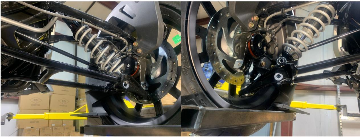
6.- Once the factory sway bar and bushings are removed, as shown below take blue painters' tape and tape up the edges of the side openings and a piece on the right as shown. Do this each side.
