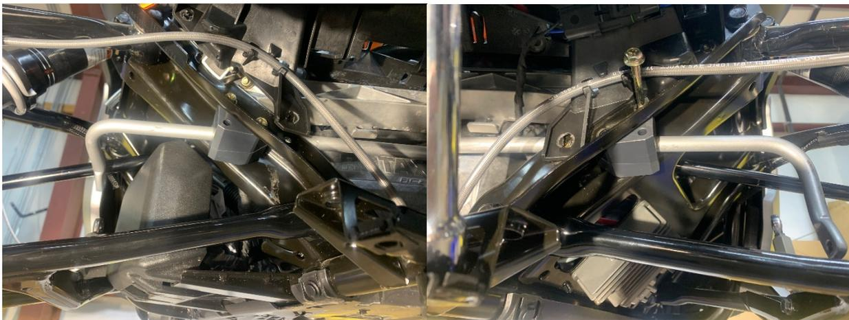
**10.- Last step is to reinstall the sway bar links to the sway bar ends. Follow the instructions for the links. Do this for both sides. Notice the bend of the sway bar is downward at the link connection.**
