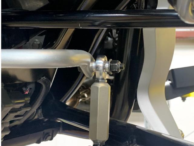
**11.-Now reassemble the Ryker in reverse of how you took it apart. Be sure to relocate the bolts in the inter plastic radiator housing. Then lower the radiator back into the position and bolt back as before. Reinstall all shock and lower a-arm bolts to the factory spec. Reinstall the Front Plastic Grille Protector and your Sway bar kits is installed.**
