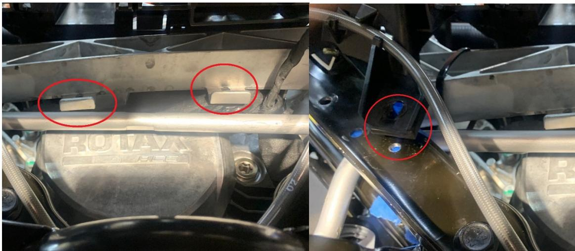
8.- Take the new way bar as shown below and run it through the left side rectangle hole. The bar should be located as shown with the end bent tabs in the upward position. With the left lower shock bolt removed it will be easier for you to allow the end of the sway bar to be moved around as shown on the lower right photo.
