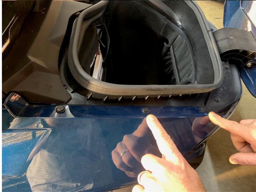
6.- Then remove the upper blue panel by pulling the panel away and sliding forward towards the front of the Spyder to release the panel.
