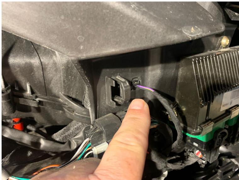
8.-Route the power wire from the docking down through the back of the steering area down through this area shown below.
