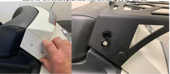
2.-Once Both mounting holes are drill each side, take the Rack and place it on the trunk as shown Above on the right-side photo. Take a rubber washer @ each hole between the Rack and Trunk then take the bolts using and plastic bolt head cover, insert in each hole then install the washer and locknut on the inside.
