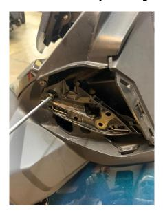
5.-Take the 3 square metal washers and 5mm carriage bolts and place them on the back side of the mirror frame mount as shown below. Then take the 3 flanged nuts and secure the bolts in place. Be sure not to overtighten. Note these are flanged nuts not the flanged locknuts.
