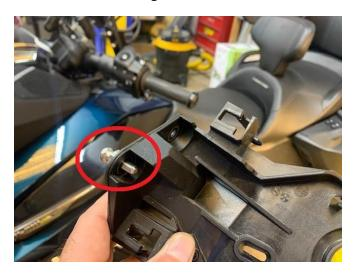
4.- Remove the Mirror Frame Bracket by removing the 4, T-20 Screws.
