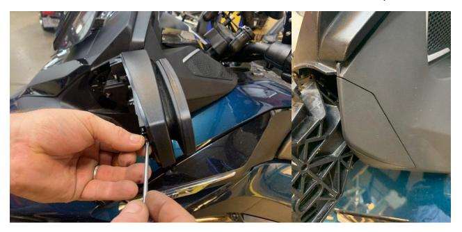
9.- reinstall the back cover and your Secure mirror bolt kit is installed. Do the same for the opposite side.
