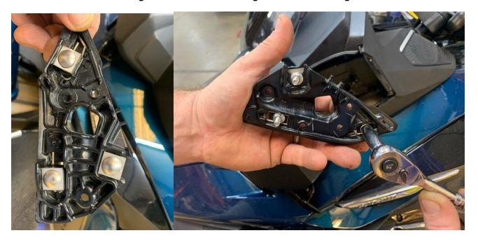
6.- Take the mirror frame mount and reinstall it in its original location and reinstall the 4 T-20 screws.
