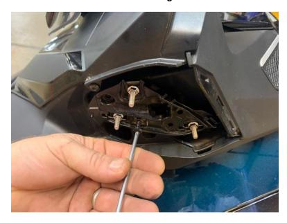
7.- Reinstall the mirror main support bracket placing it over the 3 bolts. Then apply the 3 flanged 5mm locknuts. Be sure to not over tighten.
