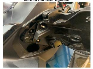
8.- Reinstall the mirror units and the T-20 screw then reinstall the front trim piece.
