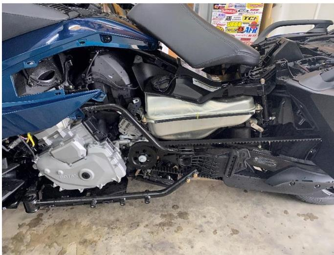
6.- Locate the two frame bolts here. Remove these bolts.
