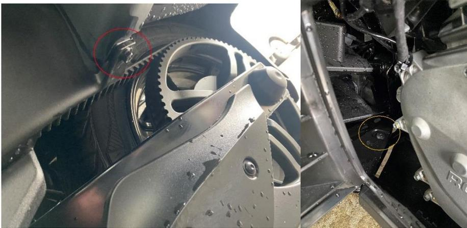
Notice these two photos of the bolt on the left underside and the screw on the right photo circled in yellow to be removed.
