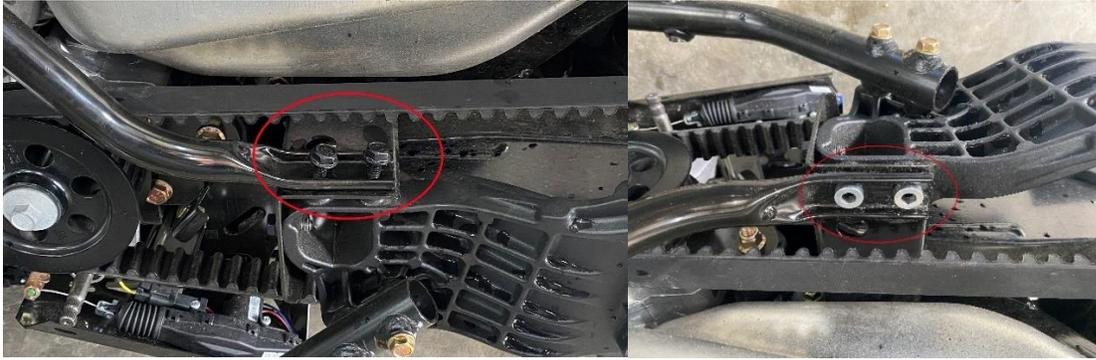
7.- Place the new belt Tensioner over the spacer. Use Blue Loctite on the new bolts. Using the new washers and bolts secure the Tensioner to the frame. **Before tightening down, the Tensioner is full adjustable, make sure the arm is parallel to the belt and the roller is centered on the belt while perpendicular to the belt. This alignment must be correct for the roller to run in alignment with the belt. Verify free motion of the arm by lifting it up off the belt.**
