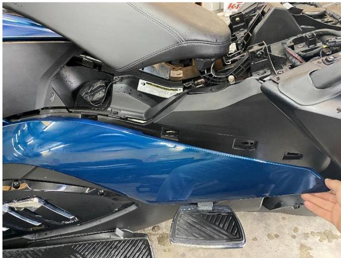
3.- Once removed next remove the driver and passenger footrest. This will make the removal of the large black panel easier without the risk of damaging it or its fasteners.
