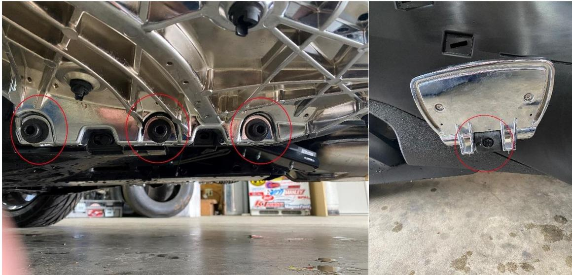
4.-Next remove the black panel the upper push pins and other bolts as shown below.
