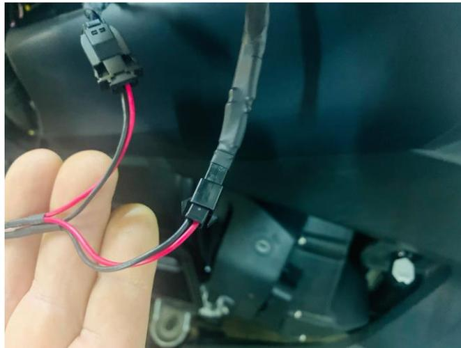
**5.- Then tie up the additional wire with supplied wire ties and reinstall the upper front cover. Make sure you leave enough wire from the Docking Station to allow the steering to move full direction each side.**
