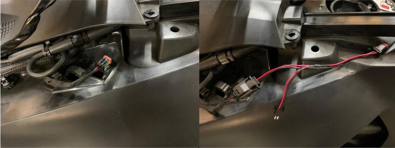
**4.- Next take the male plug form the Ryker Docking station and plug into the matching connector as this will supply the switched power to your docking station. The remaining wire end plug is for additional Ryker Factory Accessories.**
