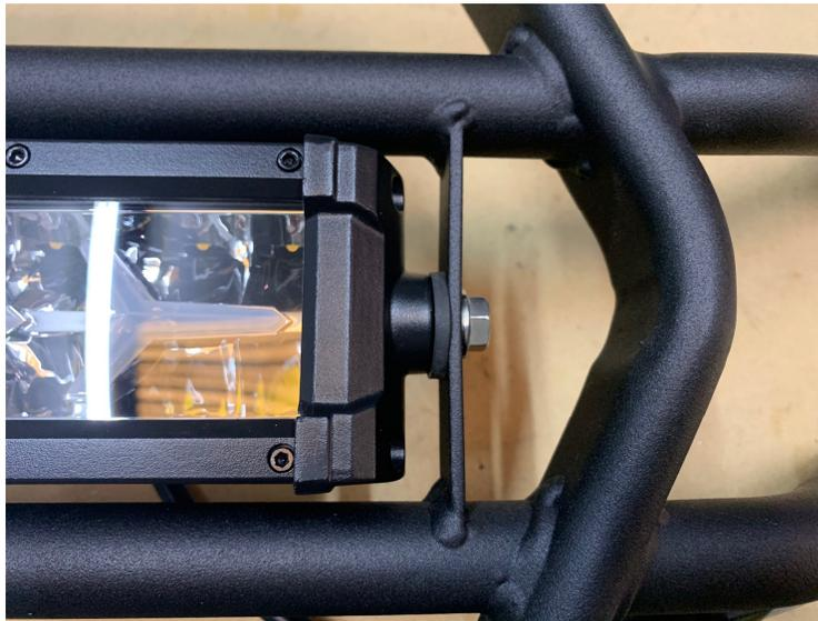
**Bolt & Rubber Washer Installed.**
