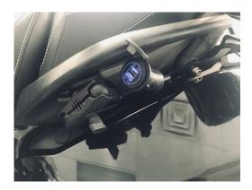
2.-The USB power unit comes two options for power depending your F3 model. If you have an F3 without the rear trunk meaning not a Limited model, under the rear passenger seat is a rubber boot with a factory fused accessory wire. You can plug the unit into the accessory wires in that boot shown in photo below. Be sure the red plugs into the positive marked wire and the black to negative.
