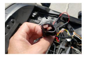
3.-The second option if you have an F3 Limited, this same rubber boot is plugged in to the trunk under the front lower side of the trunk. Simply plug the wires in the boot from the trunk and use the Y-Adapter we supply. Plug the wire adapter males terminals into the wiring hardness boot that's shown above and then the Y-Ends plug into the rear trunk wires to reconnect the trunk power and the other end of the Y-Ends to your new USB Power Dock.
