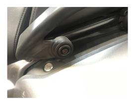
2.- Take the USB Power unit assembly and attach to the lower ball mount you just installed. As you see now you can adjust the unit to any desired position.
