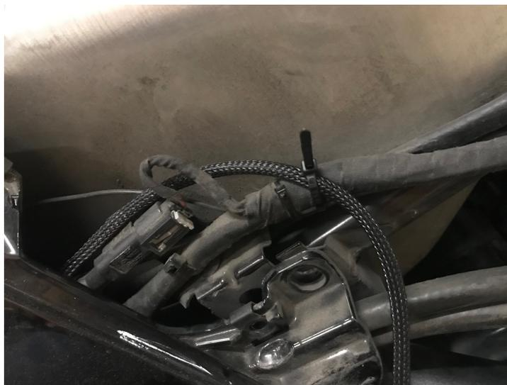
8.- Remove the left side Foot rest as you did the right side and repeat the above process. This left side LED wire is shorter, and it can be run along the inside of the panels to the upper left area access panel using wire ties as you did on the right side. Connect the Red LED wire to the other open Positive Lever Connector and the Black the same to the Negative Lever Connector
