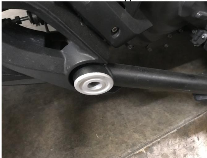
**3.-Insert the black Aluminum spacer in the front foot rest cradle as shown below.**
