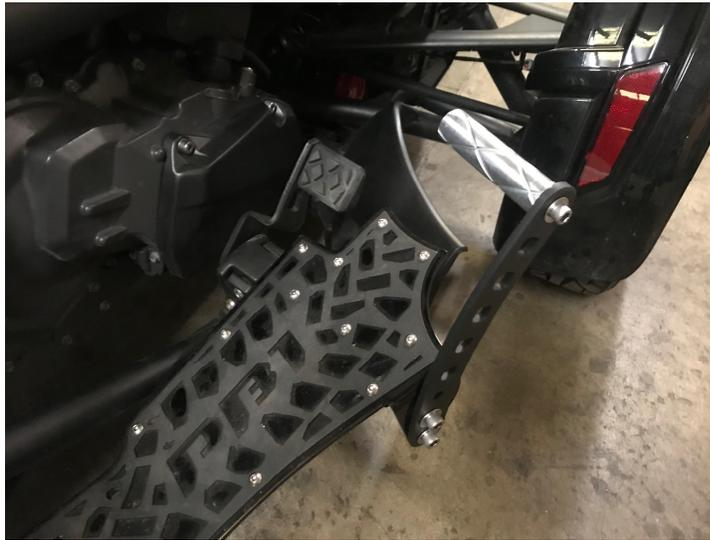
**7.- Next take the existing brake pedal pad off the brake pedal arm. Remove the two bolts from bottom side. Take the supplied spacer and new bolts and add the spacer between the brake pedal pad and the brake pedal mount. Secure using the two longer bolts.**
