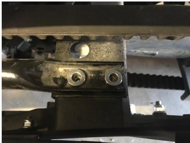
3.-Place RT Idler over the two spacers first adding the right-hand bolt and washer. With supplied new bolts, add medium strength Loctite to both bolt threads before installing. Be sure to press down on the arm at the bracket connector location to level out the mounting bracket to allow the right-hand bolt to align with frame hole. Tighten down right-hand bolt to a snug position. Then remove the 8mm alignment set screw from the left hole and replace with the bolt and washer as shown below.
